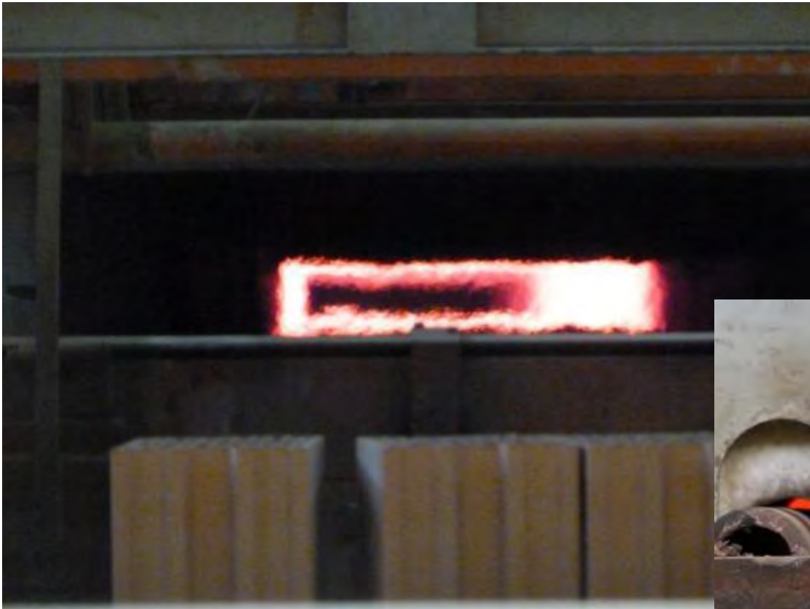
Roller kiln Firing temperature approx. 950 °C
